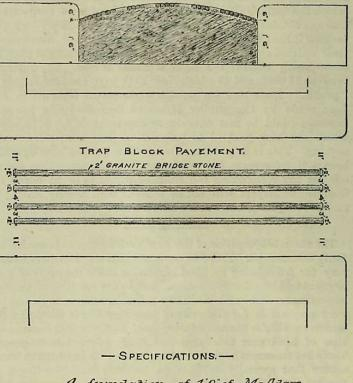
A foundation of 16 of McAdam Pavement surmounted by 4 courses of Granite Bridge stone, 2 wide and 6" deep and a Trap Block Pavement between bridge stones and curbing.
