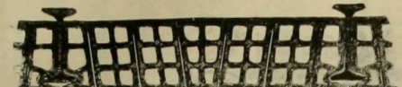
Flat arch between iron beams with skew-back protecting lower flange of beams.
