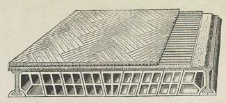
Composed of wood blocks, cemented and keyed to concrete foundation, forming a solid and immovable structure, through which no dampness or foul air can penetrate and no disease germs or filth can be secreted.
