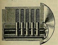
and in the adaptation of a key of sheet metal to the actuation of the peculiar tumbler mechanism shown. The original Yale lock had a perfectly flat, thin key, which was the forerunner of the innumerable forms of flat key now so generally used. It is a common mistake to characterize any lock with a flat key as a "Yale Lock," and many
