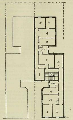
week we gave Mr. Farrington's designs for a 3-family and a 4-family tenement on a similar lot. The present design now given shows one 5-room and bath, and one 6-room and bath apartment on a floor. From all these designs enclosed shafts are omitted and open courts substituted.
