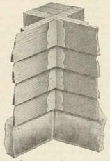
reaching clear to the corner and is then nailed on, the metal corners being applied to each course. The siding can be nailed on except at the ends and the corners slipped into place and nailed afterward if preferrd
